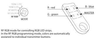
Note: The mode can be controlled by RF Touch, RF Pilot, RFWB-40/G, RF KEY, RFIM-40B, eLAN-RF-003 and
